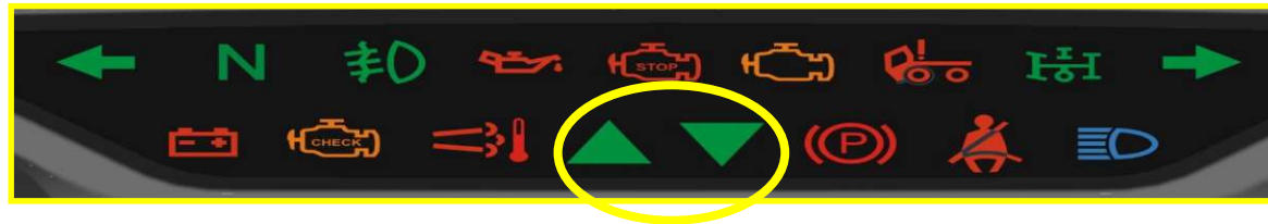
Gear Shift Advisor in Instrument Cluster
